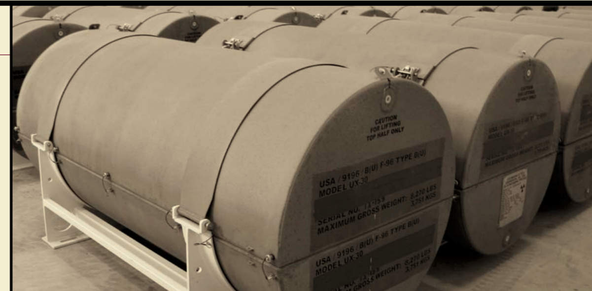
UX-30 protective covers at the site of JSC SPb IZOTOP
