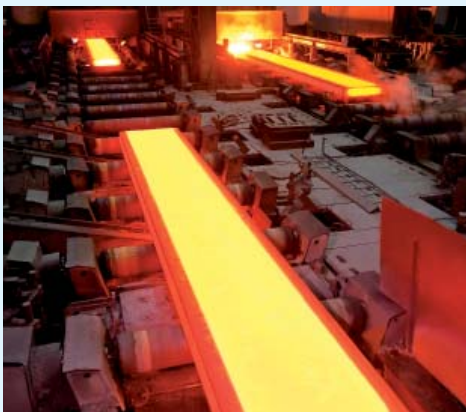
NLMK is able to produce slabs with thicknesses of up to 355 mm for further conversion into thick plate, including at NLMK's subsidiaries in Europe, NLMK DanSteel and NLMK Clabecq
