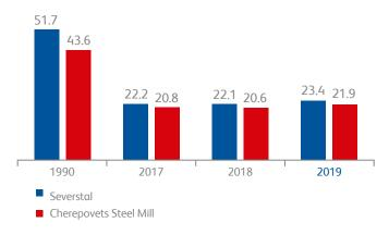
The major part of Severstal's GHG direct emissions comes from Cherepovets Steel Mill. In 2019 our overall greenhouse gas emissions increased by 6% due to the larger volume of coke production and 4% increase in hot metal output. Also, the shutdown of Turbine Generator 5 for scheduled maintenance and upgrades led to increased gas flaring.
