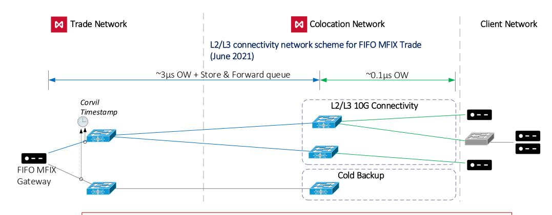
The main change is replacing single client-facing switch with a pair of <u>identical</u> switches with improved technical characteristics.
