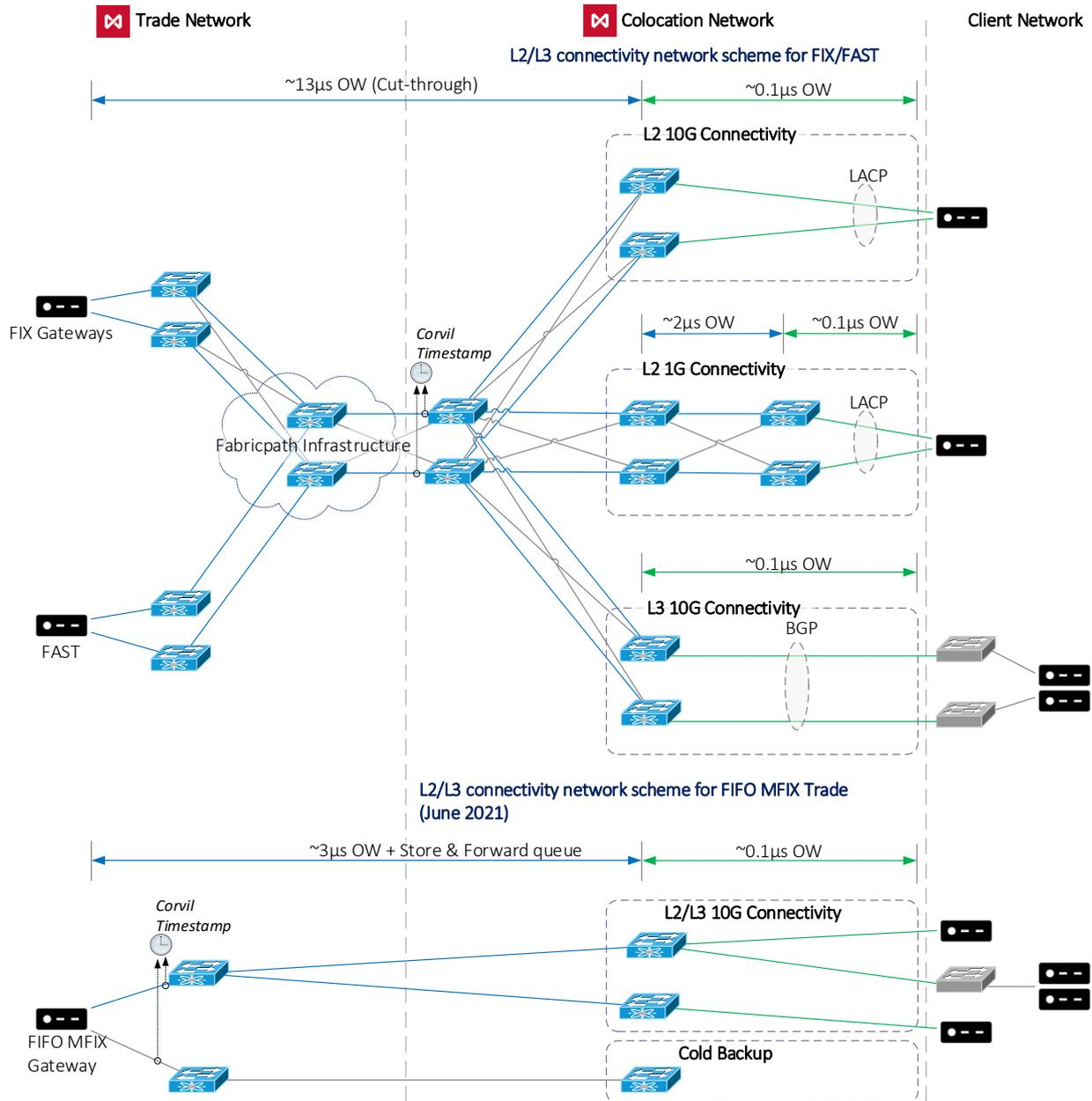
FIFO MFIX Trade network infrastructure was upgraded on 26 June 2021. The main change is replacing single client-facing switch with a pair of identical switches with improved technical characteristics.
